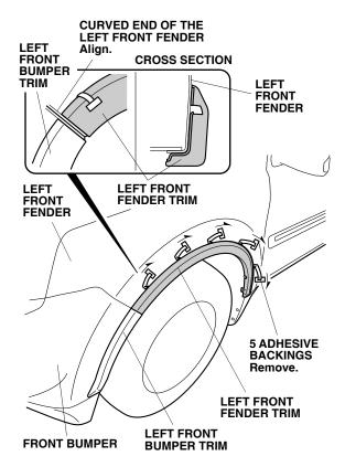
12. While applying light pressure against the left front fender trim, carefully remove the taped adhesive backings.
