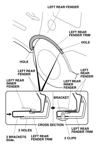
27. Install two clips to the left rear fender trim as shown.
