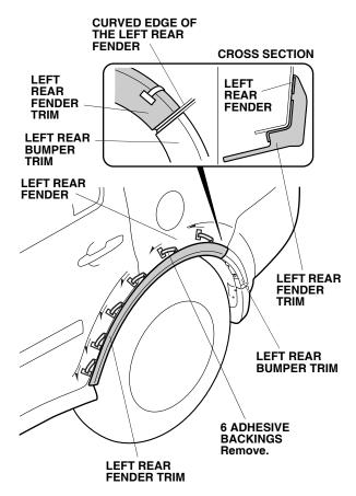
25. While applying light pressure against the left rear fender trim, carefully remove the taped adhesive backings.
