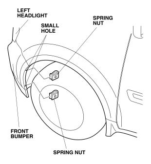
Check the fit of the left front bumper trim and the left front fender trim to the front bumper and the left front fender. Remove the left front bumper trim and the left front fender trim.
