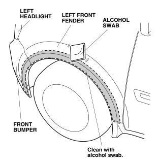
5. Peel back 1 to 1½ inches of the adhesive backing, and tape it to the front surface of the left front bumper trim. Remove the remaining adhesive backings from the left front bumper trim.
