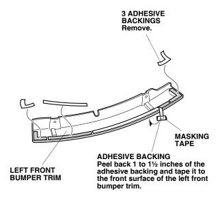
6. Align the edge of the left front bumper trim with the curved edge of the front bumper as shown. Attach the left front bumper trim to the front bumper.
