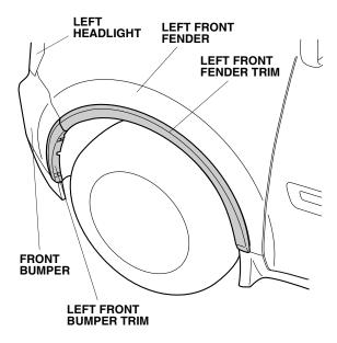
4. Using an alcohol swab, thoroughly clean the area where the left front bumper trim and the left front fender trim will attach.
