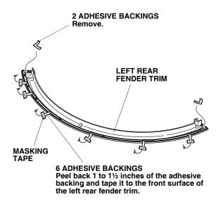
24. Align the edge of the left rear fender trim with the curved edge of the left rear fender as shown. Attach the left rear fender trim to the left rear fender.
